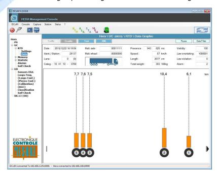
"**EICoM**" is the software used to interact with the HERA traffic analysis station.
